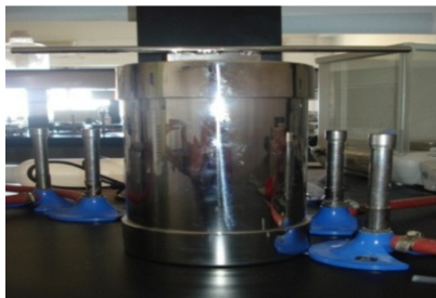
Figure 5. Pressure vessel used for heating the starch samples at 120°C.
