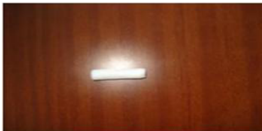
Figure 13. Starch aerogels after supercritical drying.
