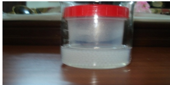
Figure 8. Na-Alginate Beads Soaked in Ethanol.
