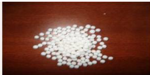
Figure 14. Na-Alginate aerogels after supercritical drying.
