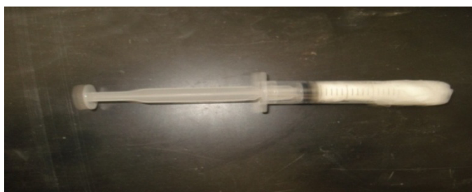
Figure 6. Cylindrical starch samples after retrogradation and aging steps.
