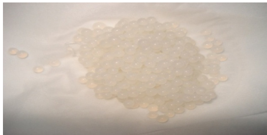
Figure 9. Na-Alginate Beads after Solvent Exchange.
