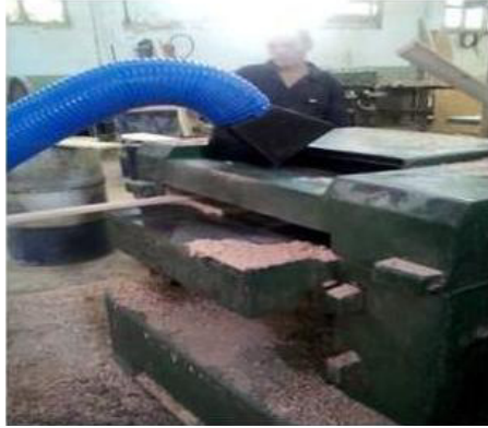
Figure 1. The system blows sawdust from the source
