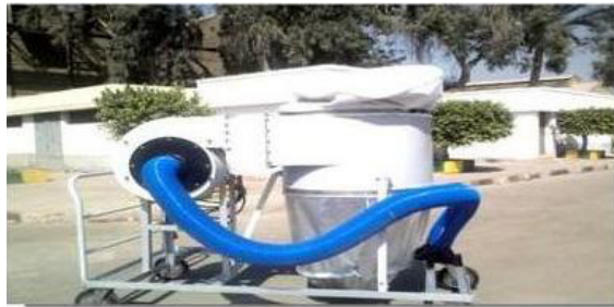
Figure 2. Our system of sawdust control
