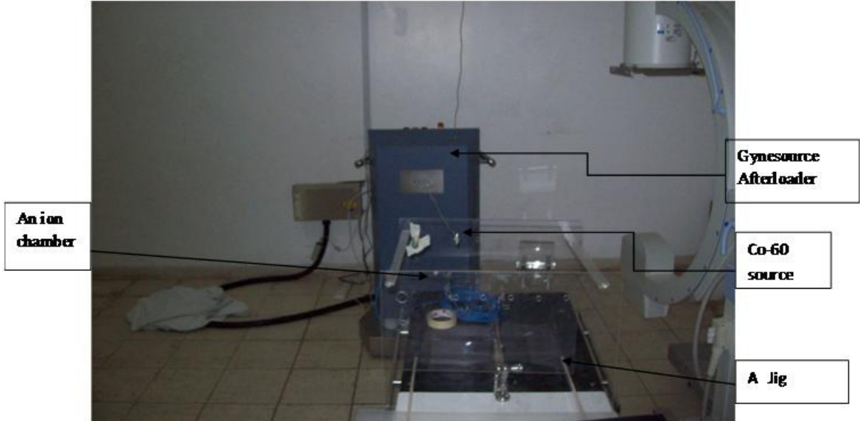
Figure 5. Set up of a jig, an ion chamber and transfer tube from the afterloader system.
