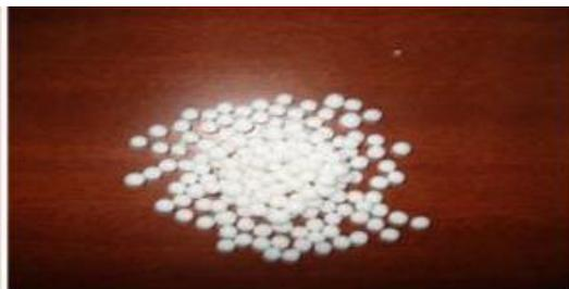
**Figure 14.** Na-Alginate aerogels after supercritical drying.
