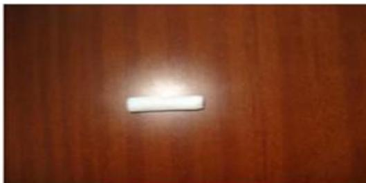
**Figure 13.** Starch aerogels after supercritical drying.
