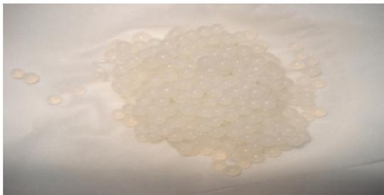
Figure 9. Na-Alginate Beads after Solvent Exchange.
